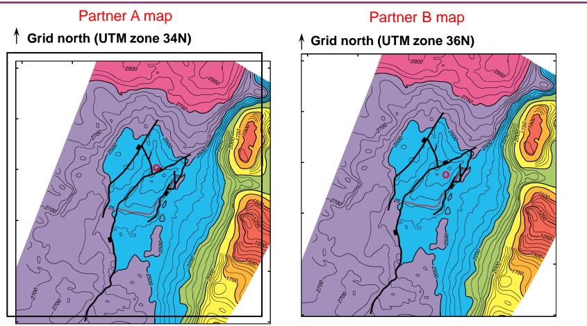
Bin grid reprojected to UTM 34N map grid. Structure now mislocated to SE. Well loc'n converted directly from lat/long coordinates Data interpreted on original CRS, well location picked at structural high. Lat/long of proposed well passed to Partner A
