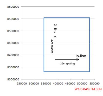
Geoscience applications require bin grids to be rectangular (have orthogonal axes) Binning the data on the acquisition projection is compliant with this
