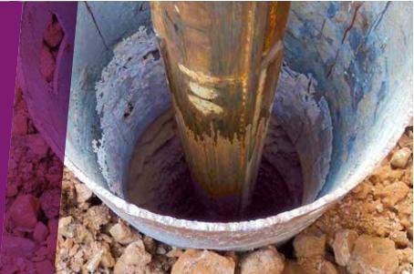
The use of acoustic tools in the evaluation of cement placement is an established practice. The measurement concept relies on an acoustic wave being transmitted along the casing and received back at the tool. The magnitude of energy loss is used to establish an acoustic coupling between casing and cement and, based on the degree of energy loss, infer the presence of cement and hydraulic isolation.
