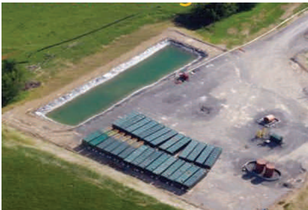
Recovered water may undergo settling in sealed tanks for later reuse. Source: courtesy of OGP members, 2014
