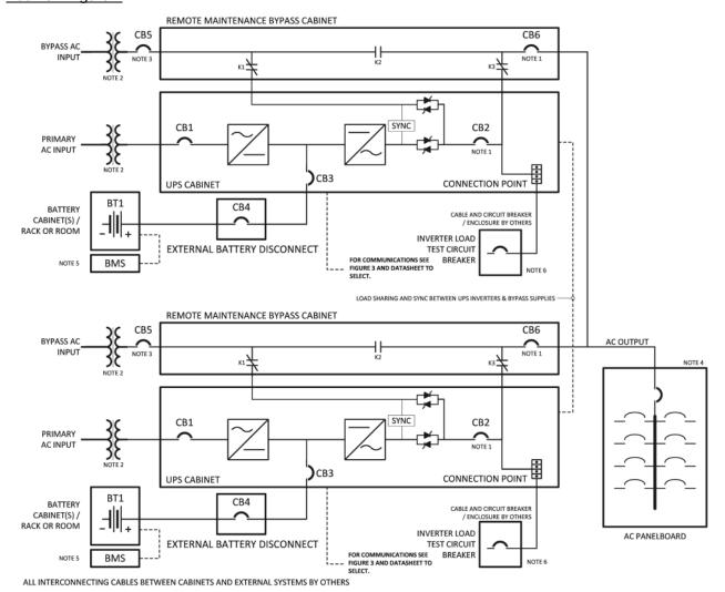
NOTE This figure is used to assist with the specification of the UPS and associated equipment. Refer to the manufacturer's literature for specific components and configuration.
