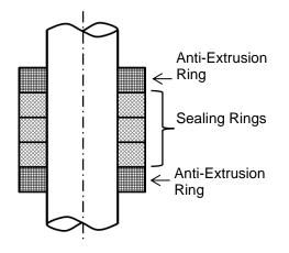
Figure 4 – Die-Formed Flexible Graphite Packing
