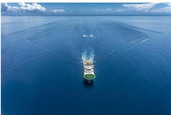
*A vessel towing a seismic array*
