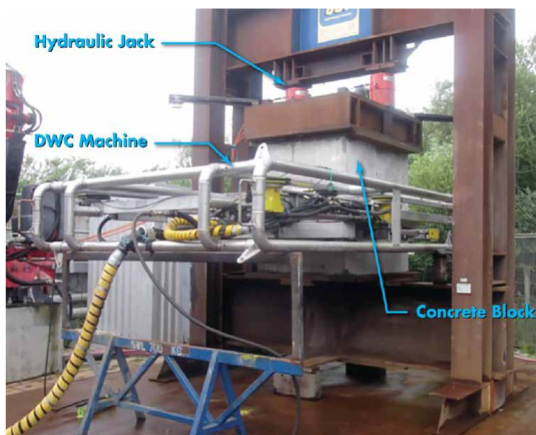
Figure 5.4: CGBS Leg Cutting Trial (Diamond Wire Cutting (DWC)) 1.2m x 1.6m test block under 500 tonnes compressive force (Photo Credit Shell).
